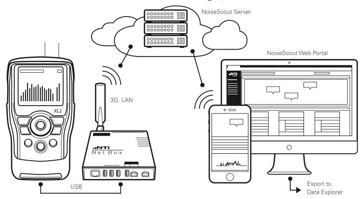
The XL2 Sound Level Meter measures the noise levels continuously and buffers all data for transmission.
